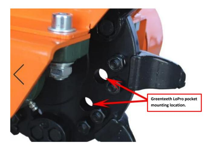
July 2020 and newer models with drilled holes allowing for fitment of Greenteeth® LoPro® Series pockets. Center spacing for pocket mounting bolts 1.53"
